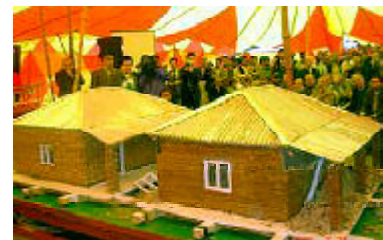
Demonstrating Shake Table using PP-Band Technology in Muzaffarabad, Pakistan
