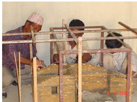
Figure 2 Workers constructing small-scale houses model for a shake-table demonstration.
