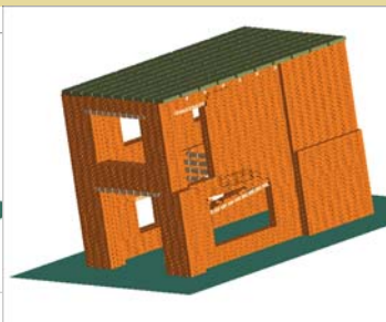
Crack pattern due to push over loading at the level of ground floor roof for building model with extra opening Assumed shear strength = 5.4 t/m 2 (minimum)
