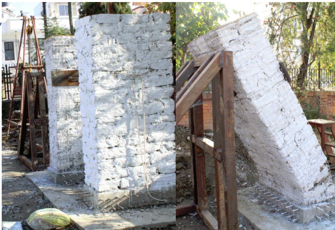
Out of plane pulldown test of stone in mud wall retrofitted using welded wire mesh
