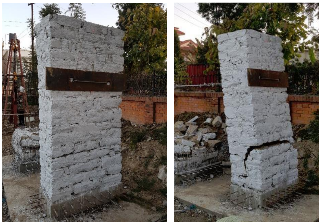
Out of plane pulldown test of non retrofitted stone in mud wall
