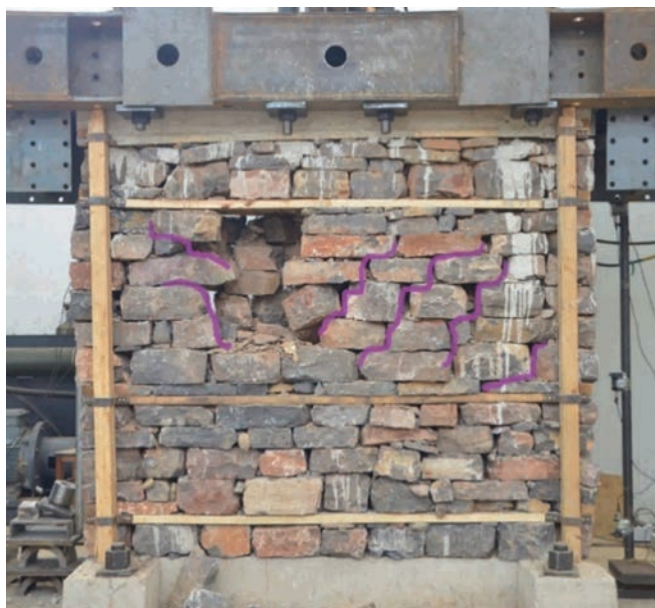
Test Set up and Wall tested on Stone in Mud with Wooden Bands
