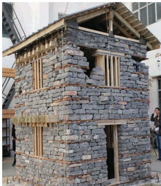
Damage to the Building with Wooden Bands and Posts as per NBC 203 at 0.51g
